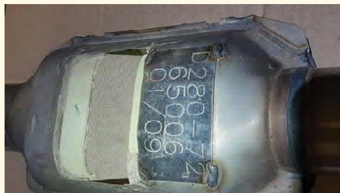
The surface area of the tiny passages within a catalytic converter that are coated with rare earth materials -- when added together -- is greater than the surface area of several football fields.
