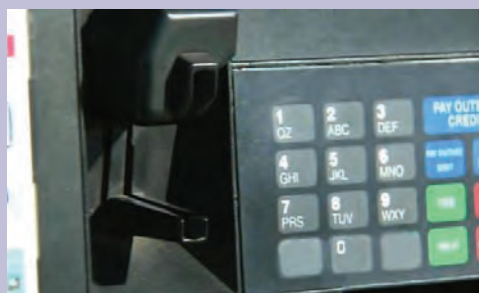
Held on with double-sided tape, the skimmer looks like any other credit card machine, just usually not quite as sturdy.
