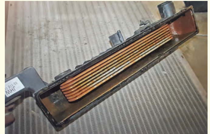
The Silverado's radiator has plastic reservoir tanks on either side of it that house the transmission oil cooler on the driver's side and the engine oil cooler on the passenger's side. Engine oil circulates through oil cooler lines into the radiator's internal engine oil cooler and the heat is transferred from the oil into the coolant.
