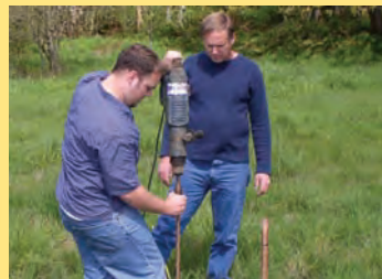
Jay Shaw, right, directs his son, Robert, in drilling the 2-foot holes necessary to place the black powder.
