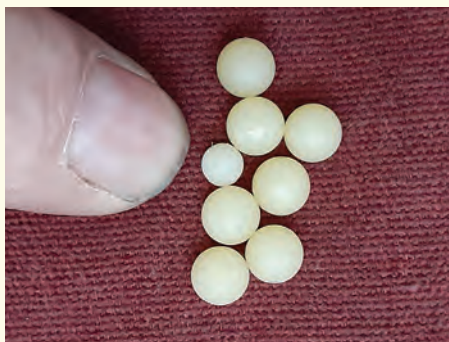
The #1 nylon check ball erodes from .250" to .180" and gets stuck in the plate passage, affecting clutch fluid supply when in drive.
