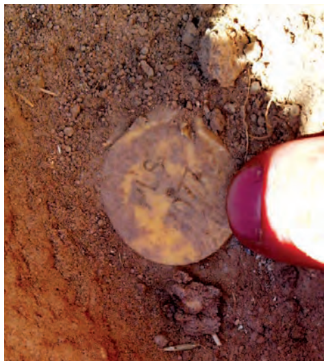
This is what they’re looking for ... a corner boundary marker. They got lucky this time since many of the 50-year-old markers are either buried, damaged or missing altogether.
