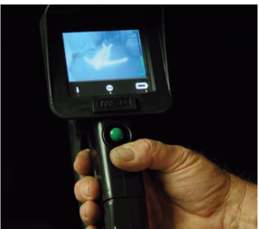
The thermal imaging camera, or TIC, allows firefighters to see through a smoke-filled room to find people or to pinpoint the source of a fire. A real lifesaver.
